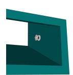
The rear chute has 2 sets of securing holes, the set required will depend on the depth of the wall. The diagram shows the set for thinner walls. Place 2 nylon washers onto each of the 2 securing bolts and loosely screw into the securing holes. Position the washers as shown.
