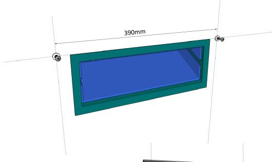
Mark the holes for the top 2 screws. These should be 390mm apart level with the top of the flange.
